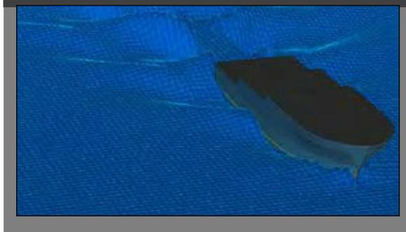
*The MAXSURF Resistance module can compute the wavemaking of slender hull shapes.*
